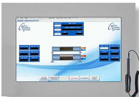
EVAPORATOR CONDENSER OVERVIEW SCREEN
